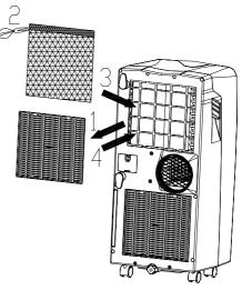
Note: Replace the activated carbon filter every 2-3 months or as needed.
